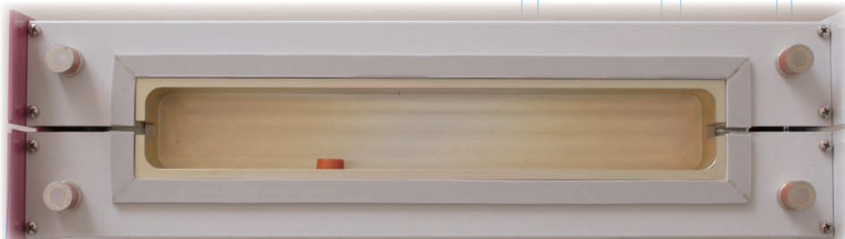
Column Chamber with Gas Sensor
